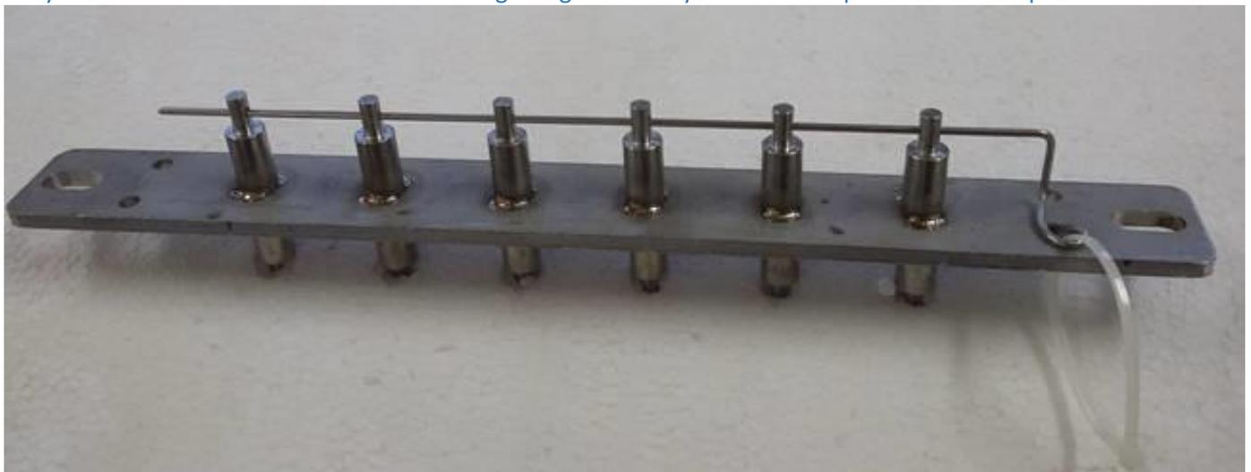
That means make an eye should be made and bend it in such way that you can fix the eye with a tyrub/cable strap through the hole in the sampler holder. See picture above and in the protocol
